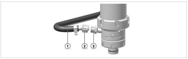
01. Tightly screw the outlet hose (1) to the outlet port (3) using the coupling nut (2).
