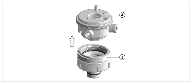
04. Unscrew the top (4) from the bottom (5) of the calibration chamber and separate the two parts.
