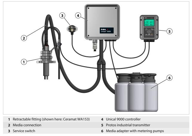
**Note:** The SensoGate WA130 may also be operated without a process analysis system. In this case, accessory ZU0631, "Standard Media Connection," is required. The SensoGate WA130 is then controlled via the process control system (PCS) or manually with accessory ZU0646, "Pneumatically Operated Manual Control Valve".  $\rightarrow$  Accessories, p. 49
