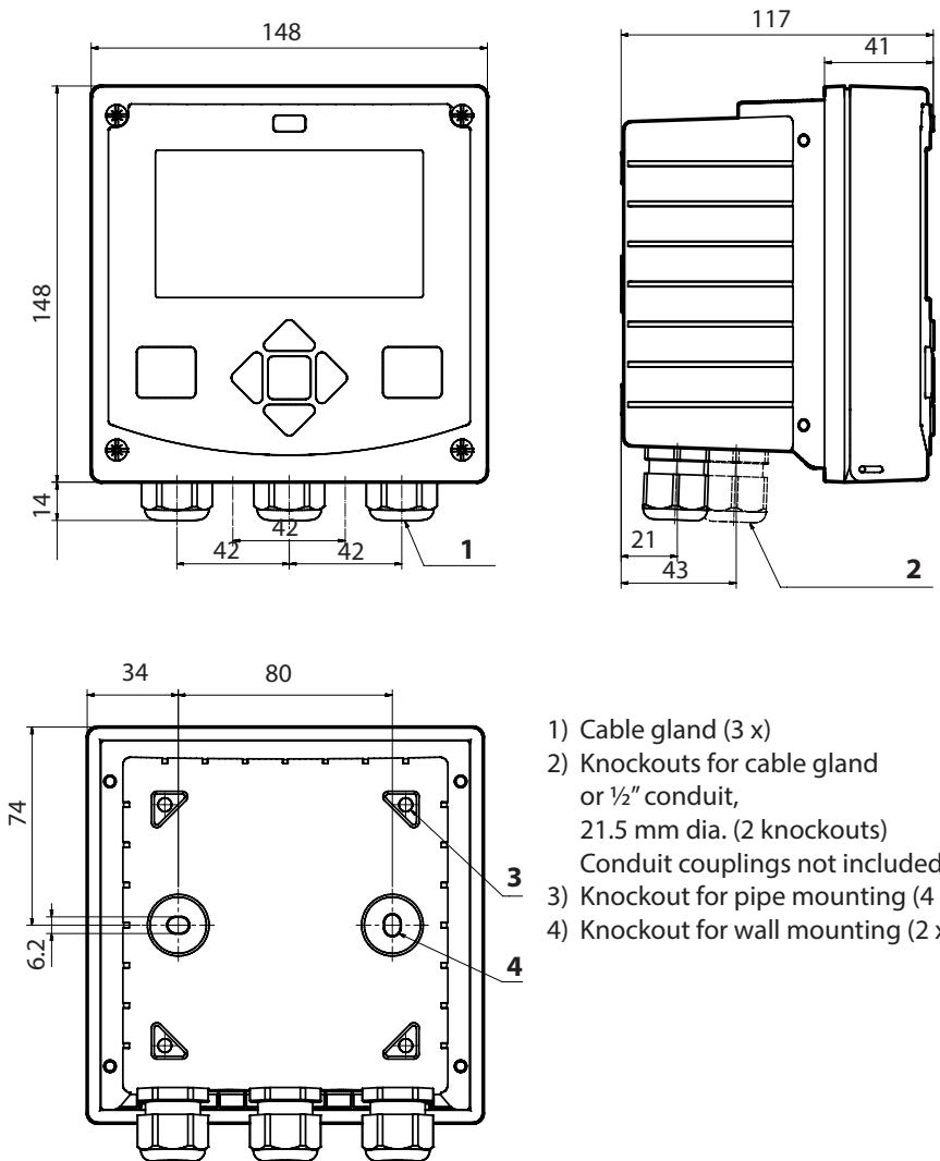
Fig.: Mounting plan (All dimensions in mm!)
