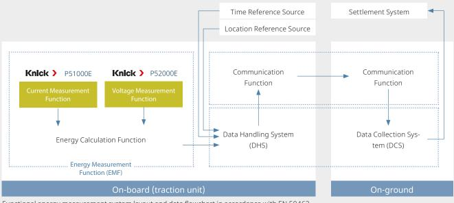
Functional energy measurement system layout and data flowchart in accordance with EN 50463
