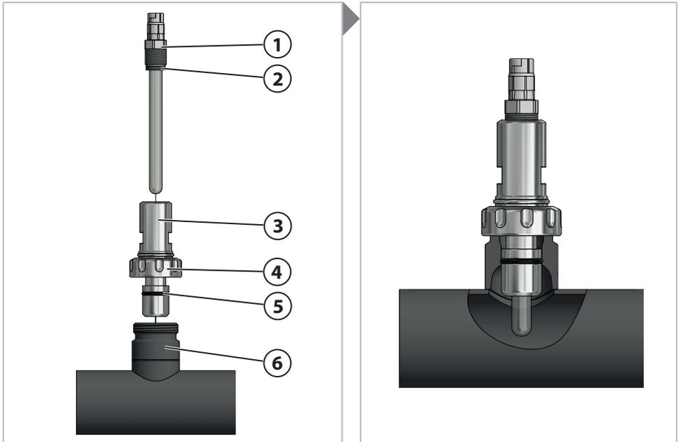
01. Check the sensor (1), thrust ring (2), and O-ring 20 x 2.5 mm (5) for damage.
