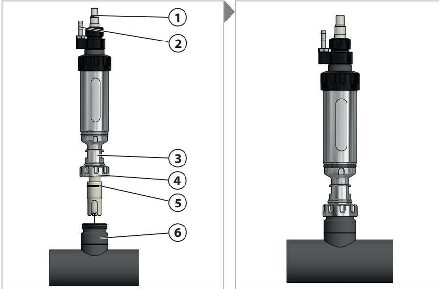
01. Check the sensor (1) and O-ring 20 x 2.5 mm (5) for damage.
