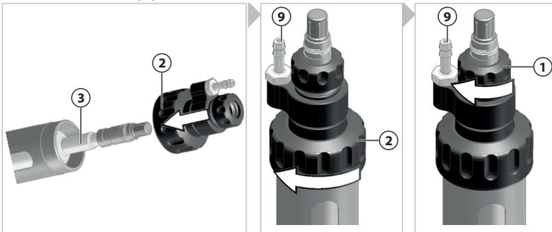
06. Position the large coupling nut **(2)** and fasten finger tight.
