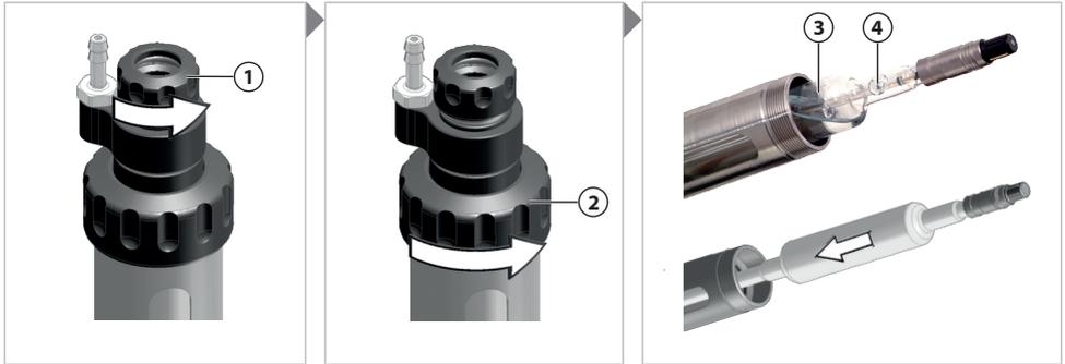
01. Loosen the small coupling nut **(1)** by a few rotations; do not loosen completely.
