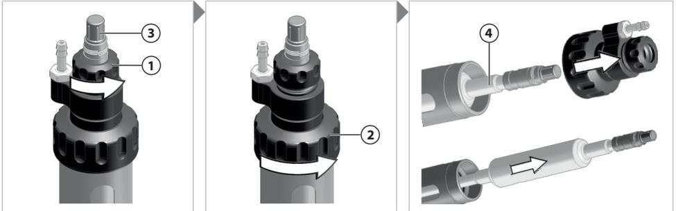
01. Disconnect the sensor cable from the sensor head **(3)**.
