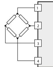
Strain gauge, internal supply (4-wire)
