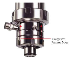
With SensoGate®, a double seal and systematically positioned leakage bores between the drive and the calibration chamber prevent control air from penetrating into the calibration chamber just as securely as they prevent the penetration of liquids into the drive cylinder. The sensor assembly drive can easily be separated from the calibration chamber by removing the union nut.
