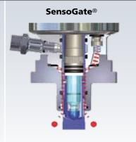
Sealing water to prevent particles being pulled in
