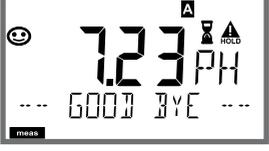
The display shows '7.23 PH' in large digits. Below it is 'GOOD BYE'. There is a smiley face icon, a 'HOLD' indicator, and a 'meas' indicator at the bottom. | After calibration is ended, the device will switch to measuring mode.                                                                                                                        | After end of calibration, the outputs remain in HOLD mode for a short time. |
