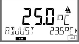
The display shows '25.0 °C' in large digits. Below it is 'ADJUST 235 °C'. There is a 'HOLD' indicator and a 'cal' indicator at the bottom.                    | Enter the measured temperature value. Maximum difference: 10 K. Press <b>enter</b> to proceed.                                                                                               | Display of actual temperature (uncompensated) in the lower display.         |
