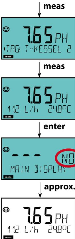
By pressing **meas** briefly you can step through further displays such as tag number (TAG) or flow (L/h). These displays are turquoise. After 60 sec they switch back to the main display.
