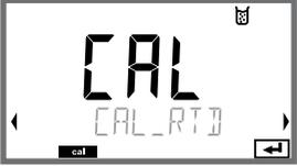
The display shows 'CAL' in large digits, with 'CAL_RT0' below it. There are left and right arrow keys and a 'cal' indicator at the bottom.                    | Select temp adjustment. Press <b>enter</b> to proceed.                                                                                                                                       | Wrong settings change the measurement properties!                           |
