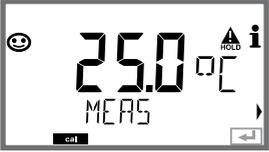
The display shows '25.0 °C' in large digits. Below it is 'MEAS'. There is a smiley face icon, a 'HOLD' indicator, and a 'cal' indicator at the bottom.        | The corrected temperature value is displayed. Sensoface is active. To exit calibration: Select MEAS, then press <b>enter</b> . To repeat calibration: Select REPEAT, then press <b>enter</b> |                                                                             |
