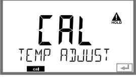
The display shows 'CAL' in large digits, with 'TEMP ADJUST' below it. There is a 'HOLD' indicator and a 'cal' indicator at the bottom.                        | Measure the temperature of the process medium using an external thermometer.                                                                                                                 | Display (3 sec)<br>Now the device is in HOLD mode.                          |
