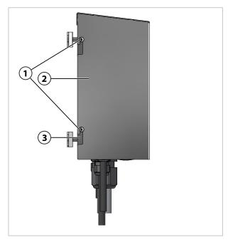
01. Loosen the screws (1) and fasten the EPC720 Cover (2) to the base plate (3) (see figure). Note: All screws are pre-installed on the base plate.
