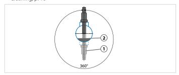
Depending on the process medium, sediments (2) may accumulate, potentially affecting the measurement result.
