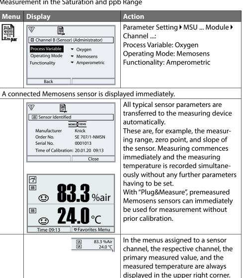
Menu Selection: Parameter Setting ▶ MSU ... Module ▶ Memosens Oxy:
