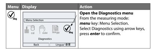
The diagnostic functions are matched to NAMUR recommendation NE 107. For a detailed description of general diagnostic functions, see the basic unit user manual.
