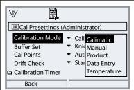
The calibration presettings can be defined in the parameter settings or adjusted directly in the Calibration menu prior to the calibration.
