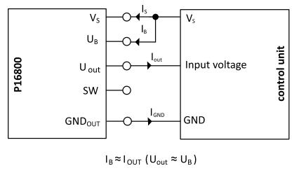
The current into terminal  $U_B$  is equal to the current that flows out of terminal  $I_{OUT}/U_{OUT}$ .
