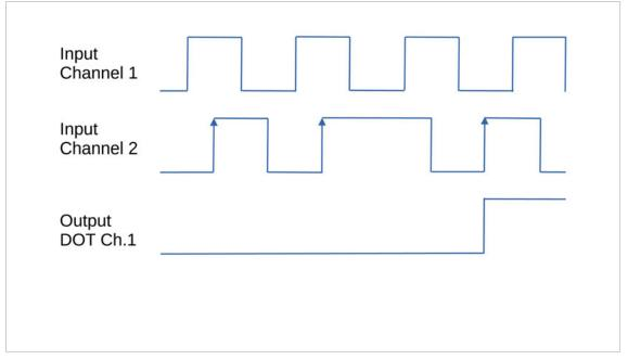
With a rising signal edge at the input of channel 2, the output level of the DOT signal is set at the output of the first channel.
