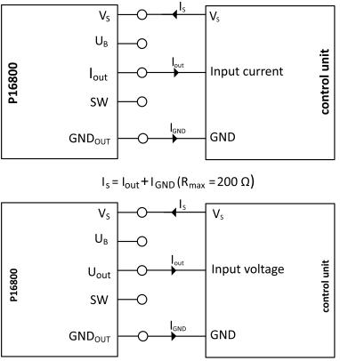
$I_s = I_{out} + I_{GND} (U_{out} \approx 4 V)$
