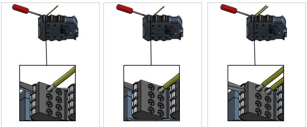
01. Insert the wire into the two-tier terminal (push-in version) without using tools. If necessary, open the two-tier terminal with a screwdriver to make it easier to insert the wire. To remove the wire from the two-tier terminal, use the screwdriver as shown.
