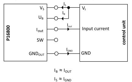
The current which flows from the controller and into the supply of the P16800, is shared as  $I_s$  for terminal  $V_s$  and  $I_{\scriptscriptstyle B}$  for terminal  $U_{\scriptscriptstyle B}$ .
