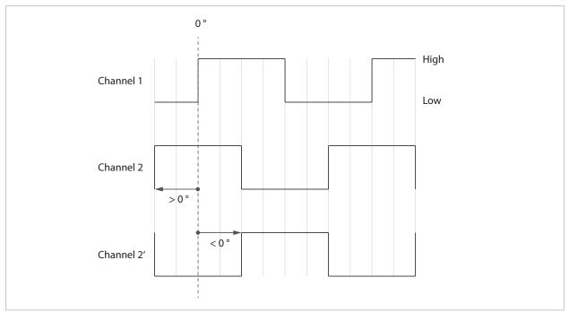
The phase shift of 2-channel speed sensors is approximately 90°.
