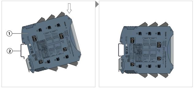
01. Snap the P16800 (1) on to the 35-mm DIN rail (2).
