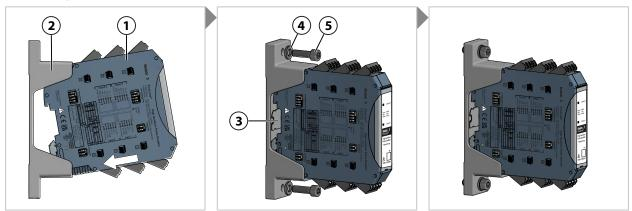
**Note:** The miniature depiction (3) on the wall-mount adapter shows the correct installation position of the P16800 (1) in the ZU1472 wall-mount adapter (2).
