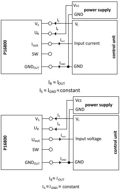
If the load on the controller is to correspond to the load through a speed sensor, an additional power supply may be used. Should the controller tolerate a higher load, the external supply source may be omitted. In this case, change the configuration of the terminal to
