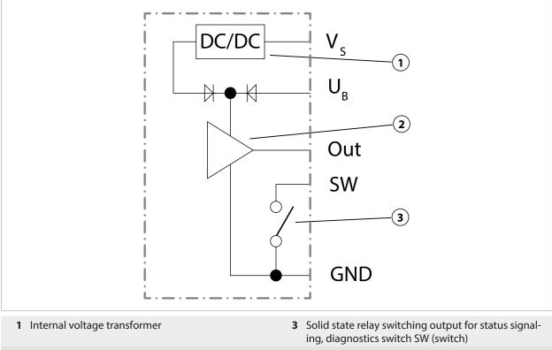
2 Output driver for current and voltage
