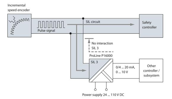
**Typical Application** – Conversion of Pulse Frequency into Analog Standard Signals
