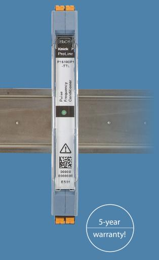
The input is designed in a way that it can "tap" signals from existing circuits without disturbing the original signal. This absence of interaction complies with the SIL 3 integrity level according to EN 61508. Even a safety-oriented signal from a sensor can be duplicated and transmitted to a second controller without any interaction.
