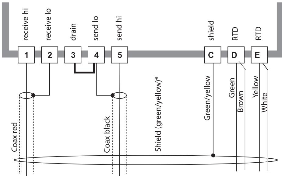
\* The shield wire (green/yellow) must be connected to the shielding mesh of the special cable using a crimp ring (see complete instruction manual, "Preparing the Shield Connection").
