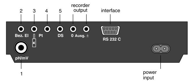
If no temperature probe is connected, the meter uses the manually selected temperature. The decimal point of the temperature display flashes.
