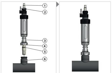
01. Check the sensor (1) and O-ring 20 x 2.5 mm (5) for damage.
