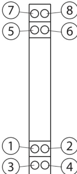
Conductor cross-section max. 2.5 mm<sup>2</sup>
