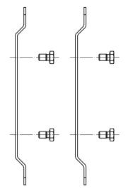
2 x wall mounting brackets (stainless steel A4) 4 x hex bolt M6x10 (A/F 10, stainless steel A4) (included in the package)
