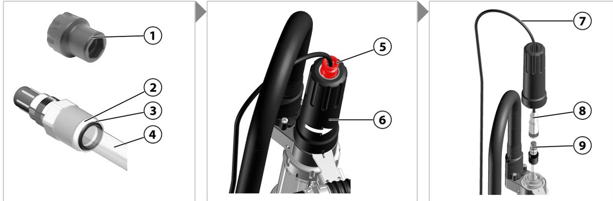
01. Move the SensoGate WA130 into the service position (SERVICE limit position).
