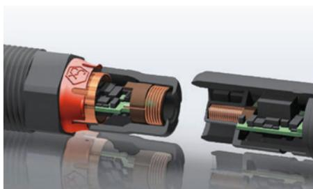
*Measured values are digitized in the sensor and transferred to the transmitter without contacts. Alongside bi-directional signal transmission, the inductive coupling supplies power to the sensor.*
