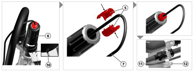
12. Attach the extension **(6)**, and turn it clockwise until the bayonet coupling snaps in.
