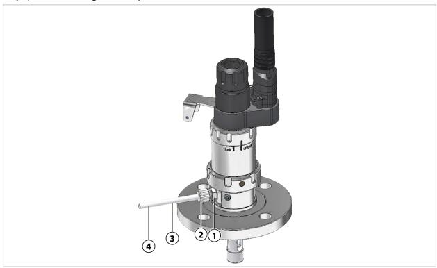
01. Tightly screw the outlet hose (3) to the outlet port (1) using the hose screw connection (2).
