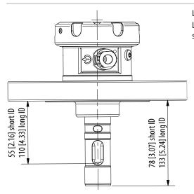
Loose flange, PN10/16, DN 32 ... DN 100 Loose flange, ANSI 316, 150 lbs, 2" ... 3" short and long immersion depths (ID = immersion depth)
