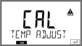
The display shows 'CAL' in large characters, with 'TEMP ADJUST' below it. A 'HOLD' icon is in the top right corner. A small 'cal' indicator is at the bottom left.                             | Measure the temperature of the process medium using an external thermometer.                                                                                                                 | Display (3 sec)<br>Now the device is in HOLD mode.                          |
