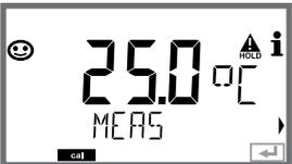
The display shows '25.0 °C' in large characters. Below it, 'MEAS' is visible. A 'HOLD' icon and an 'i' icon are in the top right corner. A small 'cal' indicator is at the bottom left.        | The corrected temperature value is displayed. Sensoface is active. To exit calibration: Select MEAS, then press <b>enter</b> . To repeat calibration: Select REPEAT, then press <b>enter</b> |                                                                             |
