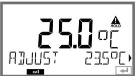
The display shows '25.0 °C' in large characters. Below it, 'ADJUST' and '235 °C' are visible. A 'HOLD' icon is in the top right corner. A small 'cal' indicator is at the bottom left.         | Enter the measured temperature value. Maximum difference: 10 K. Press <b>enter</b> to proceed.                                                                                               | Display of actual temperature (uncompensated) in the lower display.         |
