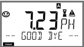
The display shows '7.23 PH' in large characters. Below it, 'GOOD BYE' is visible. A 'HOLD' icon and an 'A' icon are in the top right corner. A small 'meas' indicator is at the bottom left. | After calibration is ended, the device will switch to measuring mode.                                                                                                                        | After end of calibration, the outputs remain in HOLD mode for a short time. |
