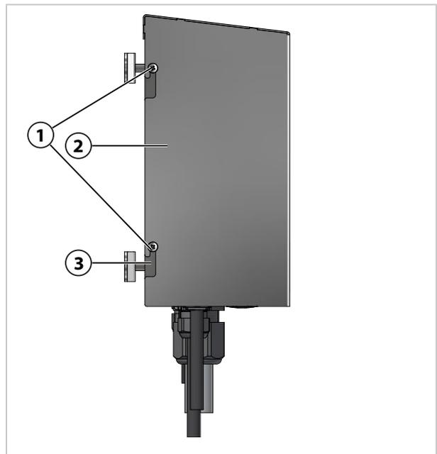
01. Loosen the screws (1) and fasten the EPC720 Cover (2) to the base plate (3) (see figure).
