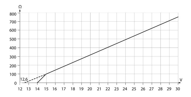
The lower voltage value in each case applies only to a load resistance of 0 Ohm.
