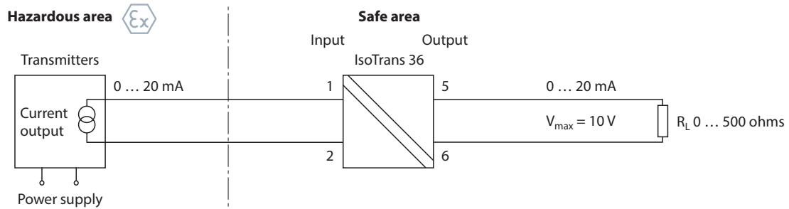
for connection to intrinsically safe current circuits with the following maximum values:
