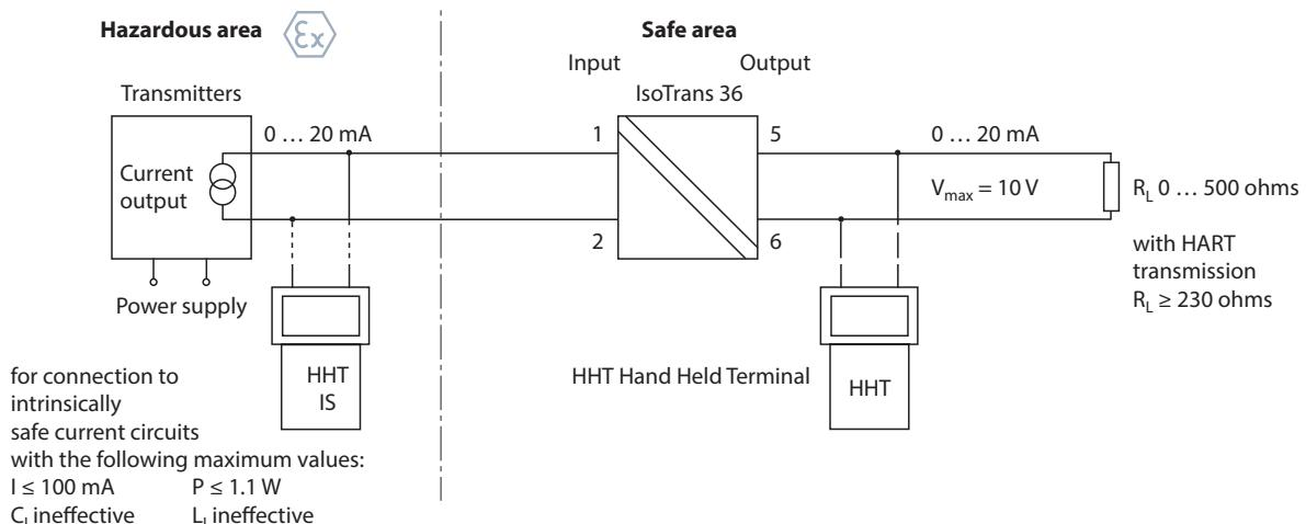
for connection to intrinsically safe current circuits with the following maximum values:
