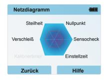
With the clearly arranged network diagram, maintenance personnel can easily read the sensor's current state at a glance.
