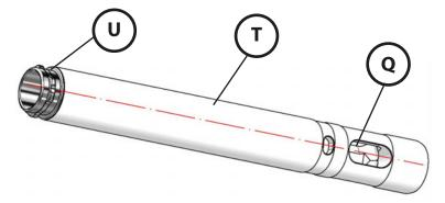
If the endpiece is not properly aligned or can be twisted, the tube is defective. In this case, you must replace the immersion tube.
