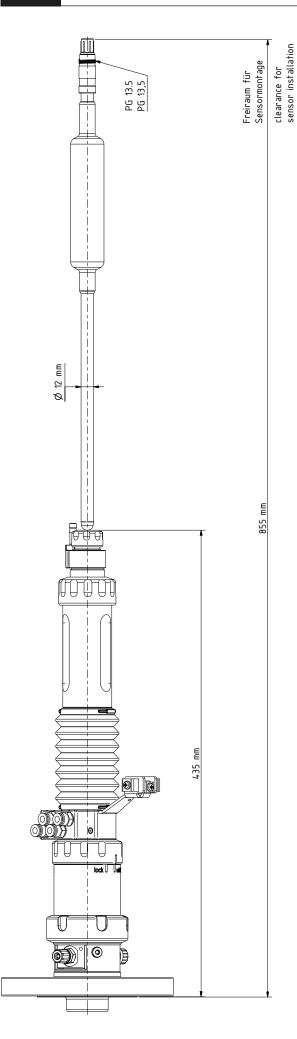
WA 133 for Sensors with Liquid Electrolyte
