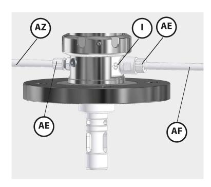
1. Connect the outlet hose (AF) using the hose coupling (AE). The outlet is marked with the following symbol (I).
