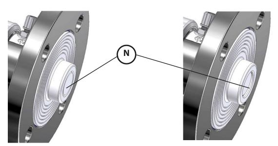
As delivered, the immersion tube fits flush with the flange bushing (N).
