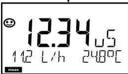
By pressing **meas** briefly you can step through further displays such as tag number (TAG) or flow (L/h). These displays are turquoise. After 60 sec they switch back to the main display.
